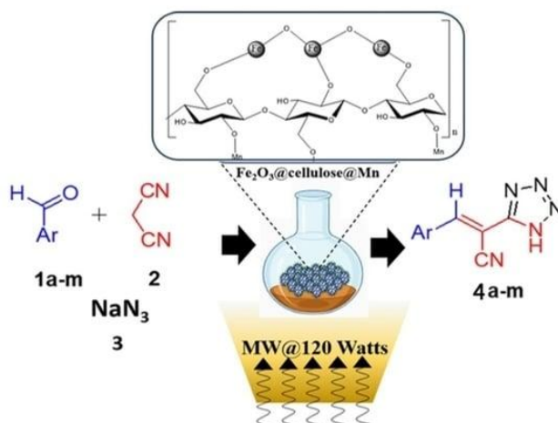
Figure 3: Role of Fe 2 O 3 cellulose Mn nanocomposite to produce tetrazole derivatives.
